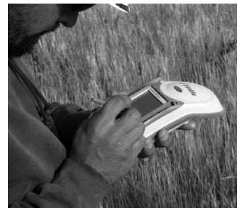
The inspector then inputs a GPS location for the pole that has been inspected.
