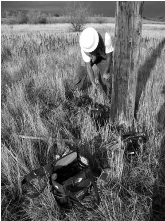
A pole inspector hammer tests a pole to ensure there is no pole rot.
