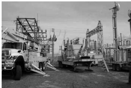
A mobile substation was brought in from Cody to be put into service if the substation could not be repaired.
